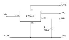
$C_1$  = Required 100 $\mu$ F electrolytic
