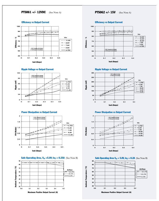
Note A: Characteristic data has been developed from actual products tested at 25°C. This data is considered typical data for the Converter. Note B: Thermal derating graphs are developed in free-air convection cooling, which corresponds to approximately 40–60LFM of airflow.
